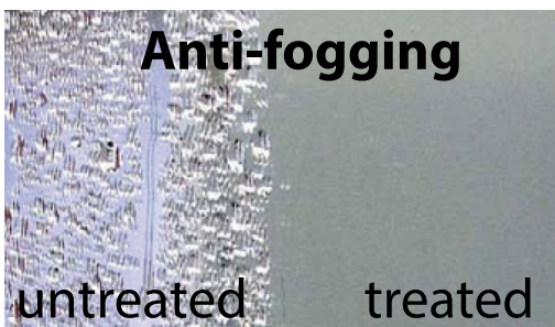
1- ProClean Image applied to 1 tile, half treated half untreated.
